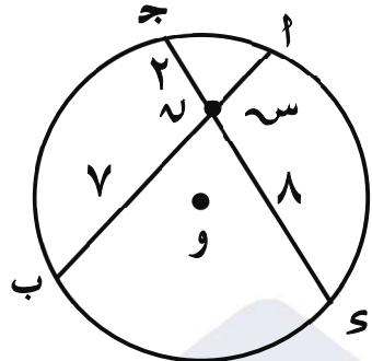
$$\begin{aligned} أ \times ب &= ج \times د \\ س \times ٢ &= ٧ \times ٨ \\ \frac{٦٣}{٧} &= \frac{٦٤}{٨} \\ س &= \frac{٦٤}{٧} = ٢,٢٨٥ \end{aligned}$$
