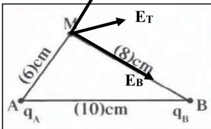
$$E_A = \frac{Kq_A}{d^2} = \frac{9 \times 10^9 \times 3 \times 10^{-8}}{(0.06)^2} = 75000 \text{ N/C}$$
