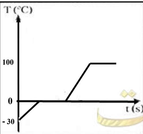
$$Q_1 = c_{ice} m \Delta T = 2090 \times 0.1 \times (0 - (-30)) = 6270 \text{ J}$$
