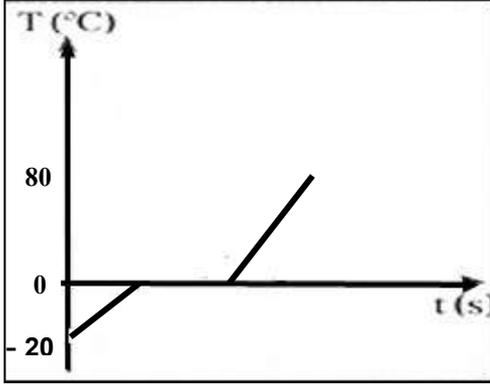
$$Q_1 = c_{ice} m \Delta T = 2090 \times 0.2 \times (0 - (-20)) = 8360 \text{ J}$$
