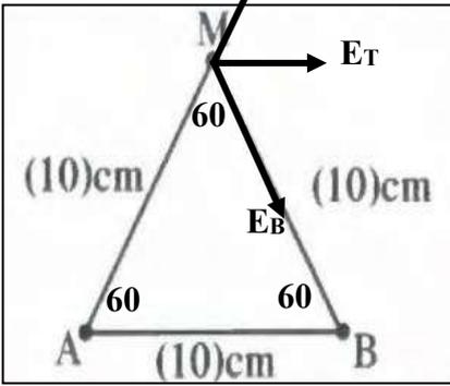
$$E_A = \frac{Kq_A}{d^2} = \frac{9 \times 10^9 \times 2 \times 10^{-8}}{(0.1)^2} = 18000 \text{ N/C}$$
