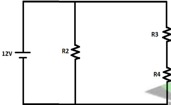
$$R_{eq1} = R_3 + R_4 = 5 + 5 = 10 \Omega$$
