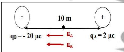
$$E_A = \frac{Kq_A}{d^2} = \frac{9 \times 10^9 \times 2 \times 10^{-6}}{(5)^2} = 720 \text{ N/C}$$
